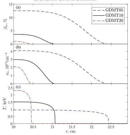
FIGURE 4. Radial profiles of the warm plasma (a) relative pressure, (b) density and (c) temperature outside the bubble core  $r \ge a$  for the regimes GDMT05 (blue dashed curves), GDMT10 (black solid curves) and GDMT20 (red dash-dotted curves) specified in Table 1.
