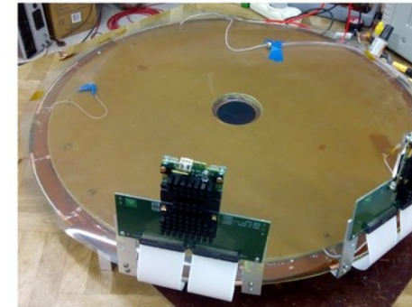
muRWELL at the jig for gluing
