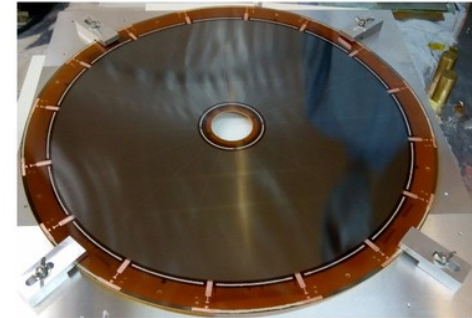
muRWELL at the jig for gluing
