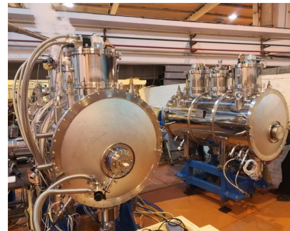
Assembling of 54-pole indirect cooling 3.5 Tesla wiggler for KSRS, (March 2019)
