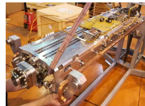
Assembling of 54-pole indirect cooling 3.5 Tesla wiggler for KSRS, (March 2019)
