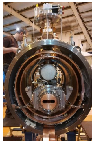
Assembling of 54-pole indirect cooling 3.5 Tesla wiggler for KSRS, (March 2019)
