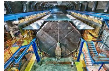
Far Detector 735 km from beam target 5.4 kton mass
