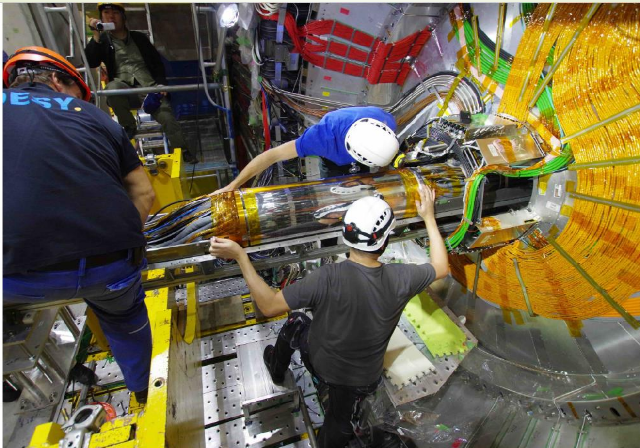
Figure 96. Photo taken during the VXD installation in the Belle II detector: installation of the VXD in the Belle II detector. The slide guide installed in the Belle II detector using the slide guide installed in the forward part of Belle II.
