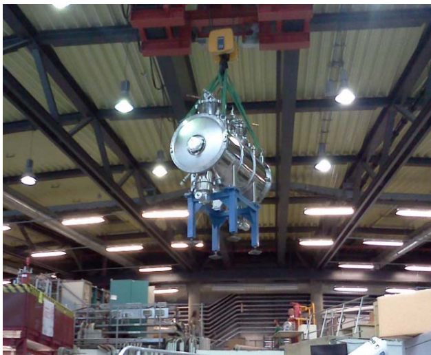
Fig. 6.5.4. Transportation of the upgraded 7 T HMI (HBZ) wiggler to the BESSY-II storage ring.
