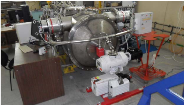
Fig. 5.6.3. Vacuum pumping system.
