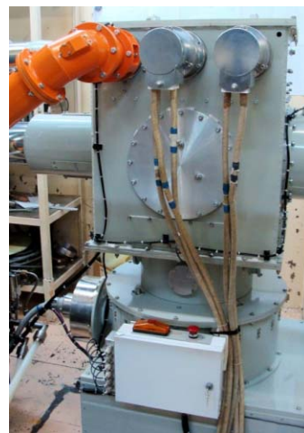
Fig. 7.15.1. Left: – transistor preamplifier and pre-output stage on GU-92A; right: output stage on GU-101A.
