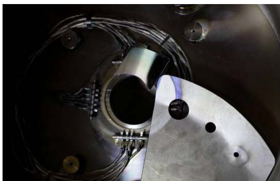
Рис. 9.1.6. The imprint of argon beam on a rotatable diaphragm located at the entrance of the H^- beam into the accelerator.
