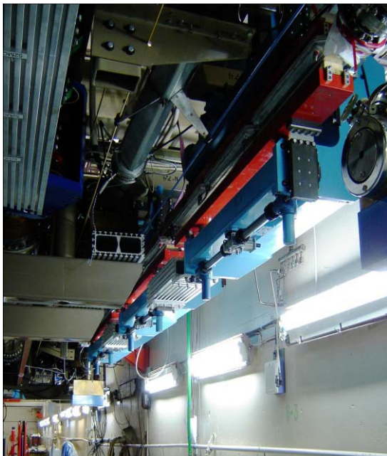
Fig. 6.4.6. Undulators of the third stage of the FEL on the fourth track of the ERL.
