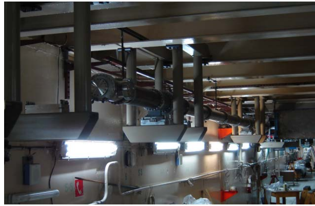
Fig. 6.4.3. Vacuum chamber of the optical cavity of the third-stage FEL, suspended in the accelerator hall.
