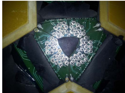
Fig.1.3.1: Photo of 60-channel photodetector based on CPTA 151-30 silicon photomultipliers.
