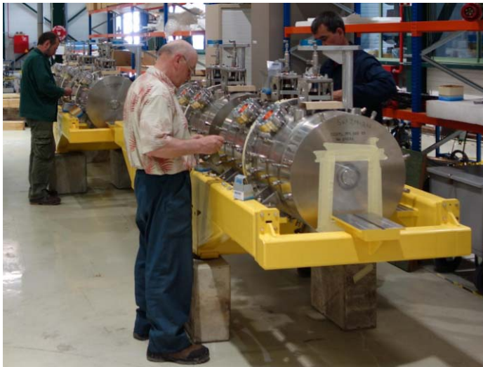
Fig. 7.9.4. Left: preparation of CCDTL modules 5 and 6 to tests at CERN. Right: module 2 secure bunker during "hot" tests.
