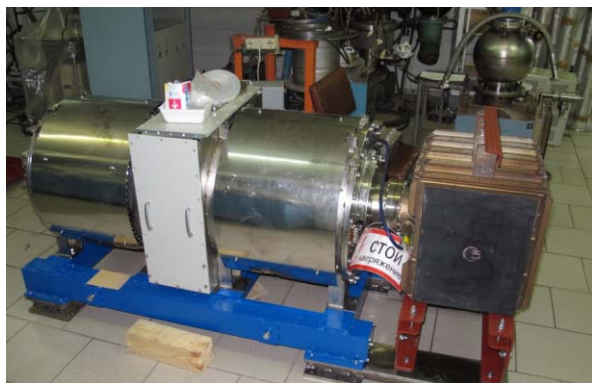
Fig. 7.10.1. Cavity with attached ion pump.
