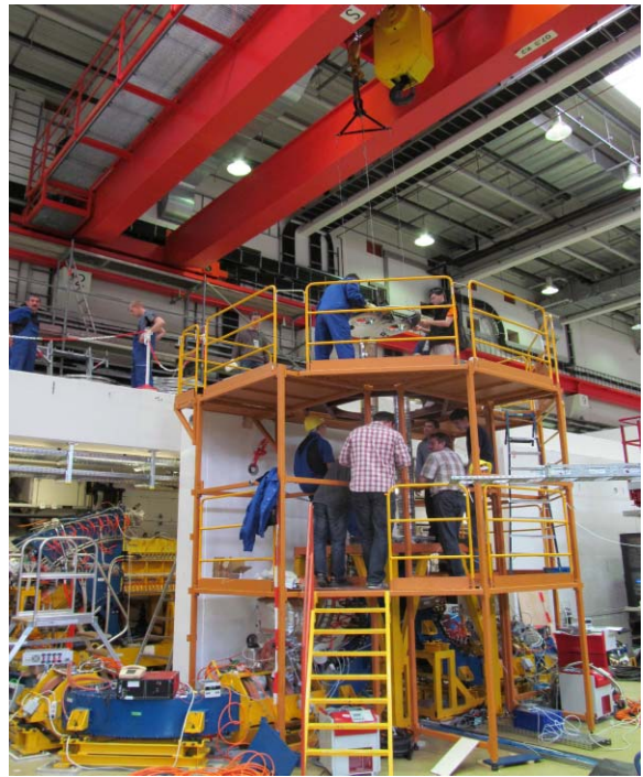
Fig. 5.9.2. Assembling the electrostatic accelerator in Germany.
