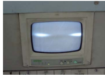
Fig. 5.2.5. Image of the electron bunch with energy of 1.85 GeV on the SR monitor at the RF voltage amplitude on the plates of about 6.5 kV.
