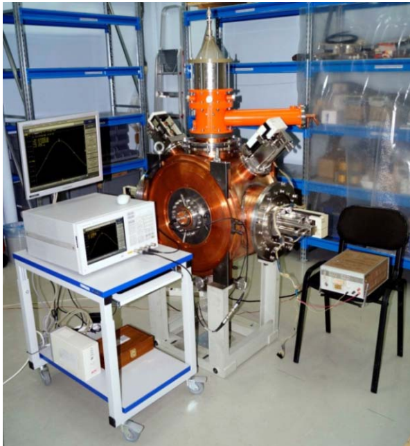
Fig. 7.5.1. RF measurements of parameters of the new BEP cavity.
