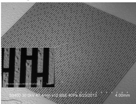
Fig. 6.2.11. SU-8 resist micro-lattice on glass-carbon substrate with gold plating about 50 microns thick. The period of the structure is 130 microns; the line width is 65 microns; the total field of the lattice is 1 \times 1 \text{ cm}^2 .
