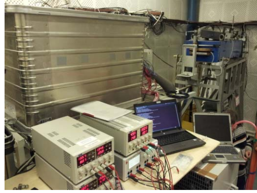
Fig.1.3.3 Photo of FARICH prototype with DPC on extracted electron beam.
