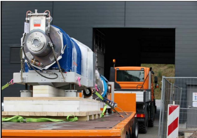
Fig. 5.7.3. Transport of first SHF stations to the building of the XFEL injector.
