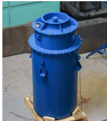
Fig. 6.4.4. New high-voltage rectifier for the electrostatic electron gun.
