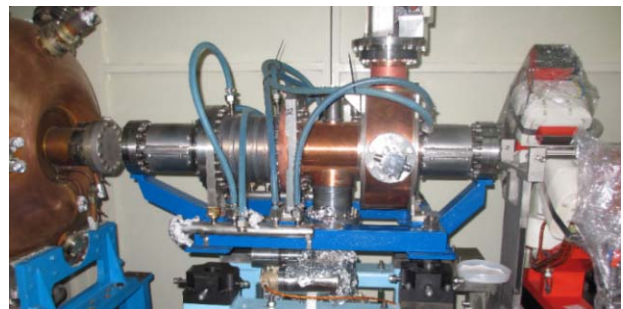
Рис. 7.6.1. Passive single-mode cavity mounted on the storage ring at National Synchrotron Radiation Laboratory, Hefei city, China.
