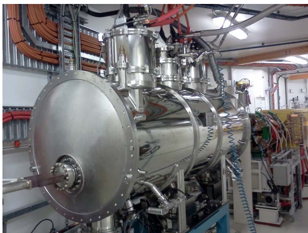
Fig. 6.5.1. 63-pole 4.2 T wiggler with period 52 mm, installed on the storage ring of the Australian Synchrotron (AS) in Melbourne for biomedical research.
