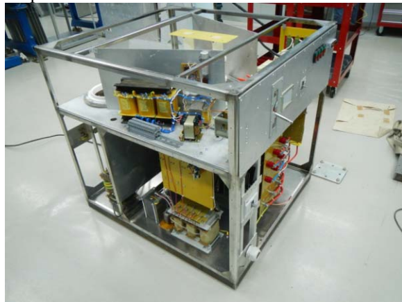
Fig. 7.10.2. RF power amplifier during mounting.
