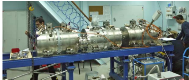
Fig. 7.9.3. Accelerating CCDTL module during vacuum tests at BINP.
