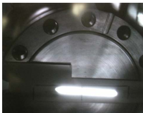
Fig. 6.3.7. Synchrotron radiation of the 8 th beam line from the 7-pole wiggler in the SR bunker of VEPP-4.
