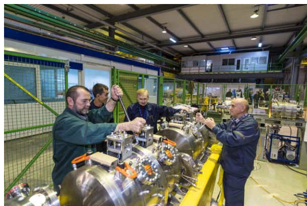
Fig. 7.10.2. BINP team assembling CCDTL module 2 at CERN.
