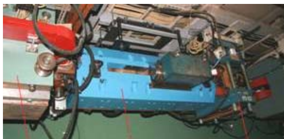
Fig.5.2.4. 7-pole wiggler with a 3T field, installed in the northern semi-ring of the VEPP-4M accelerator.
