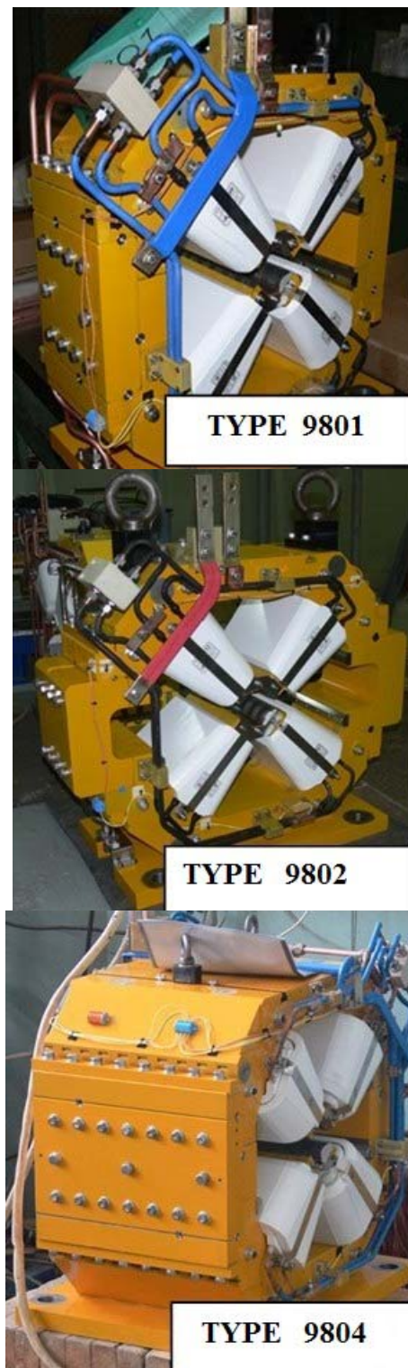
Fig. 5.6.1. Types of the BINP lenses for the main ring of the NSLS II synchrotron radiation source.
