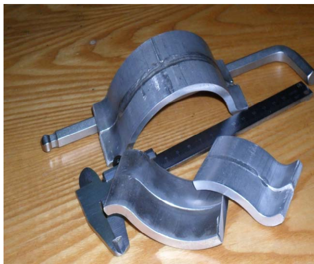
Fig. 5.4.3. Vacuum chamber fragments welded on the stand for electron beam welding.
