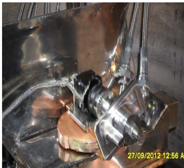
Fig. 5.4.2. Four-drive system with stepper motors.
