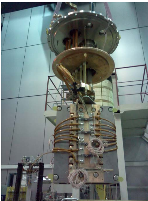
Fig. 6.5.5. Prototype of the superconducting helium-free wiggler CLIC with a 3 T field for the ANKA storage ring (Karlsruhe, Germany).
