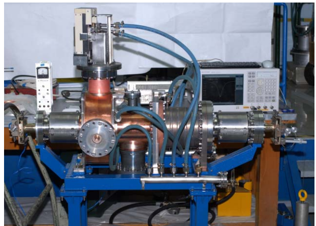
Fig. 7.7.1. 816 MHz single-mode passive RF cavity.
