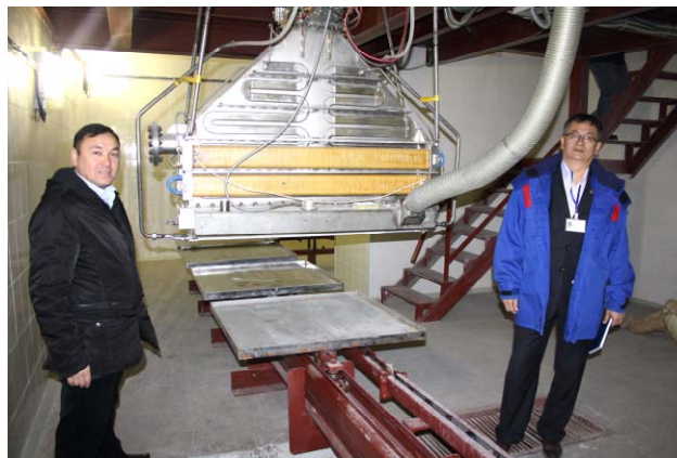
Fig. 8.2.2. Modernized beam extraction device with the new beam scanning system and the underbeam conveyor, ILU-10 machine, Kurchatov, Kazakhstan
