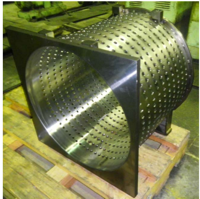
Fig. 7.11.5. Housing of half cavity with openings for cooling air.
