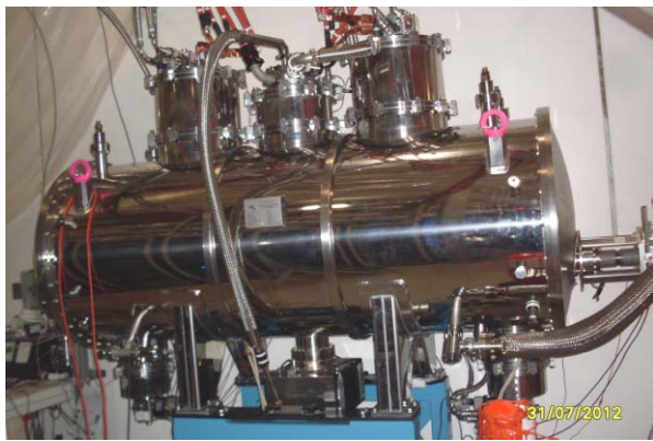
Fig. 6.5.1. 63-pole 4 T wiggler for the Australian Synchrotron storage ring (Melbourne).
