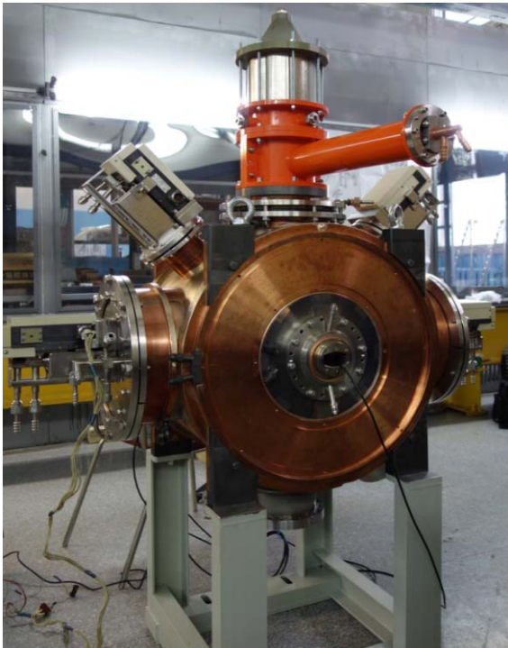
Fig. 7.6.1. New BEP cavity during check assembly in the experimental workshop.
