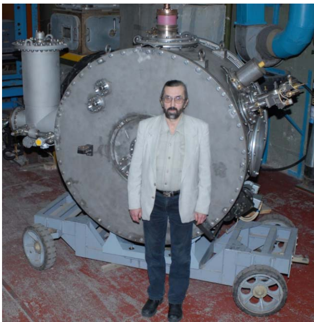
Fig. 7.8.1. 181.8 MHz cavity after the rework.
