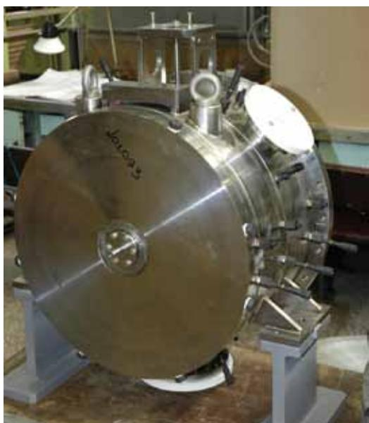
Fig.(7.13)4. The body of the cavity of the 1st module is prepared for vacuum tests.
