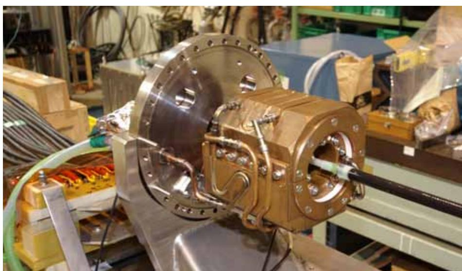
Fig.(5.13)2. Pulsed magnet for the positron source of the KEK Super-B Factory.
