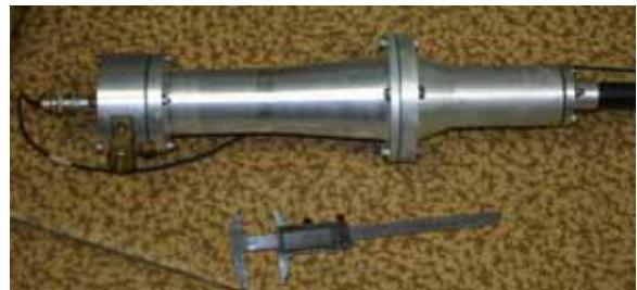
Fig.(5.14)1. Thyratrons TPI1-1k/35 and TGI1000/25 and a 50 ohm load (from left to right).
