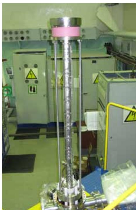
Fig.(5.11)1. Drift structure of MIS-1.
