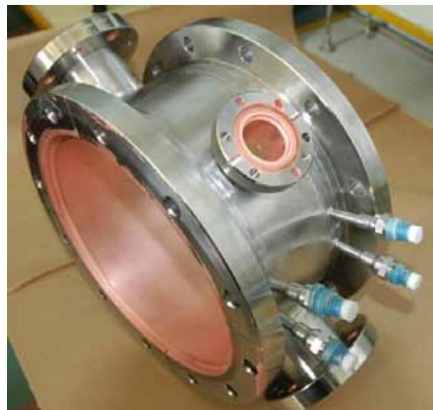
Fig.(7.13)5. Coupling cell of the 1st module after application of the copper coating.
