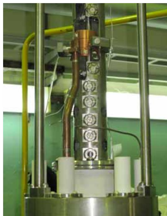
Fig.(5.11)2. System for dosed injection of atoms of solids and the inner part of the gas system.
