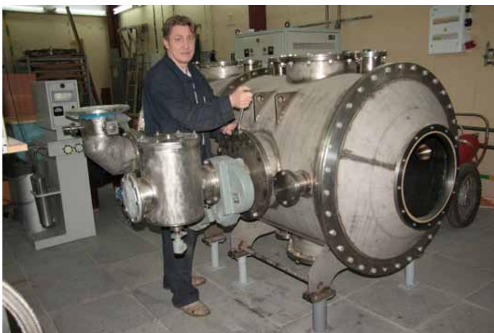
Fig. (5.5)5. Vacuum chamber of welding facility which develop in frame of ISTC project “Development of vacuum system and production technology for high luminosity electron – positron colliders”.
