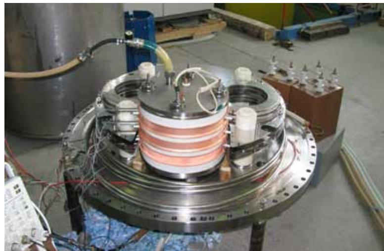
Fig.(5.7)2. Transformer section under testing.
