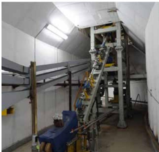
Fig. (5.3)6. Elements of downtake channel to VEPP – 3 with coolant circuit.
