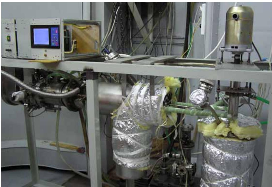
Fig. (5.5)4. Welding gun on the shielding window test stand with liquid lead.
