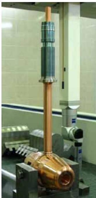
Fig.(7.13)2. Pilot sample of the drift tube.
