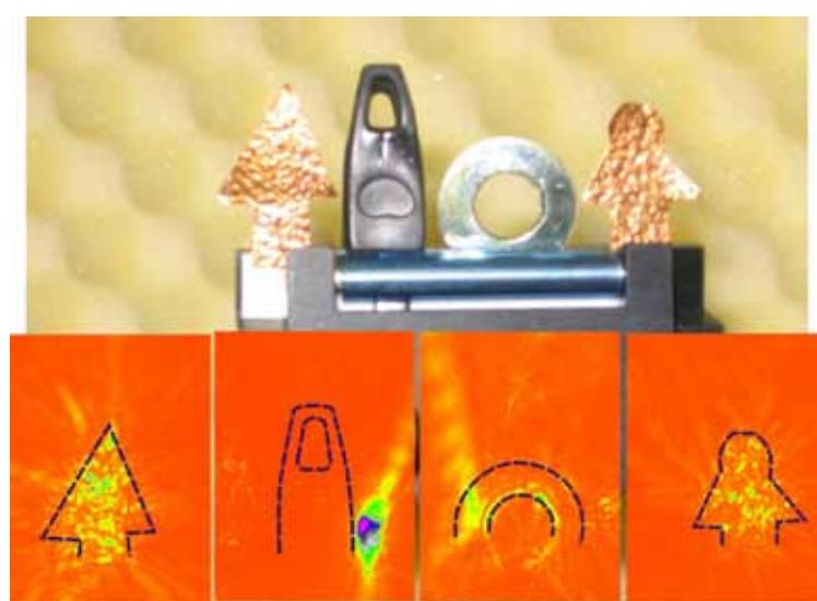
Fig.(6.3)12. Images of objects in the terahertz region, taken with the Fresnel lens and a microbolometer array.
