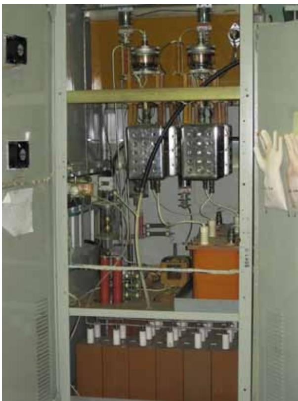
Fig.(5.11)3. Anode modulator.
