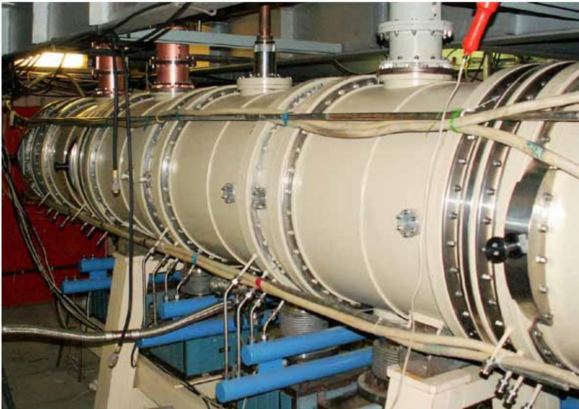
Fig.(7.5)6. Accelerating structure after matching of the power inputs.
