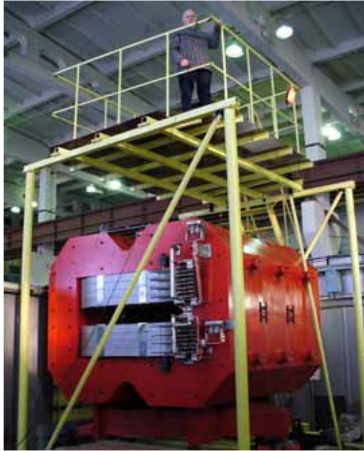
Fig. 37: Radiation-resistant dipole magnet of the H type.
