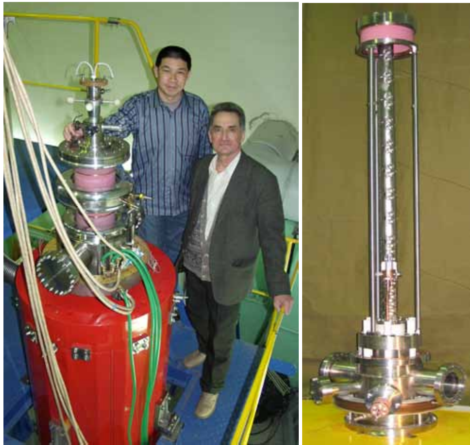
Fig. 2. MIS-1 (left) and its drift chamber (right).
