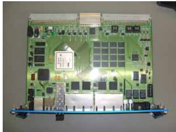
Fig. 4. The electron module of the 16-channel shaper-digitizer in VME standard and the electron module of the concentrator in VME standard.
