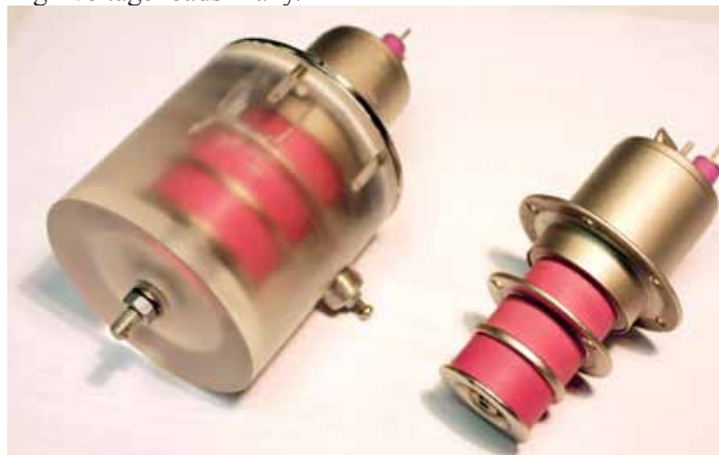
Fig. 3. The TPI-1K-35 pseudo-spark switch with the isolating housing filled with a carbogel (up to 40 kV) and without housing (up to 20 kV).
