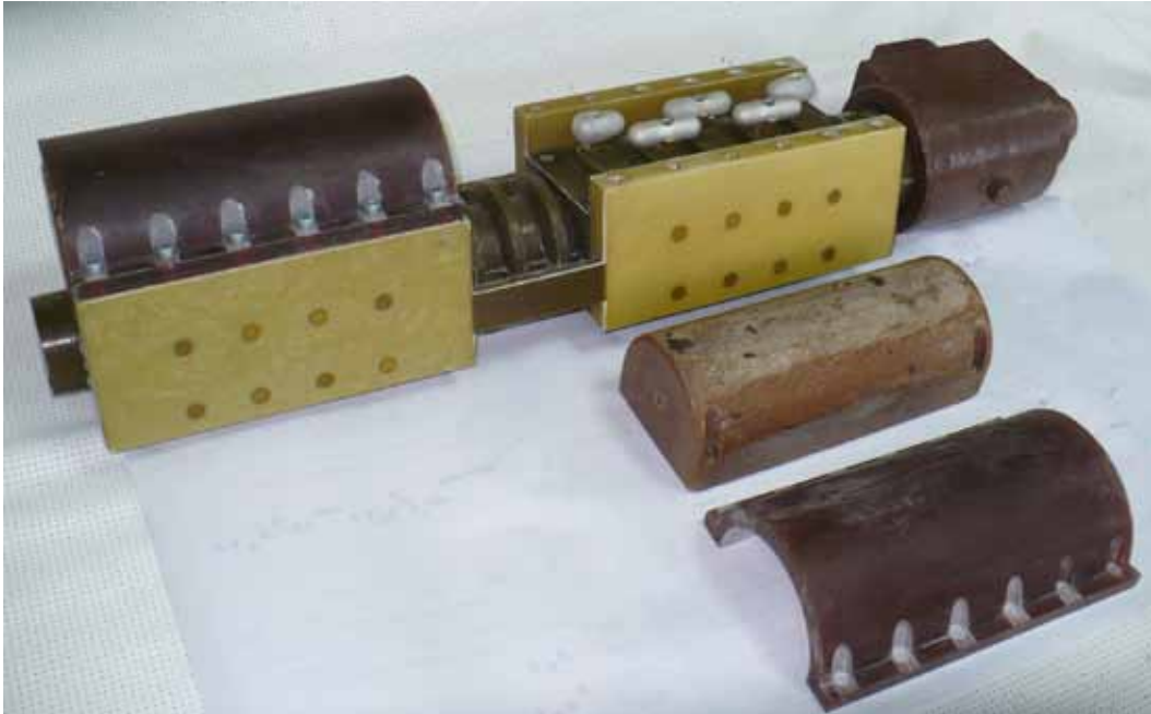
Fig. 13: Photo of the high-current discharge switch, manufactured at BINP.
