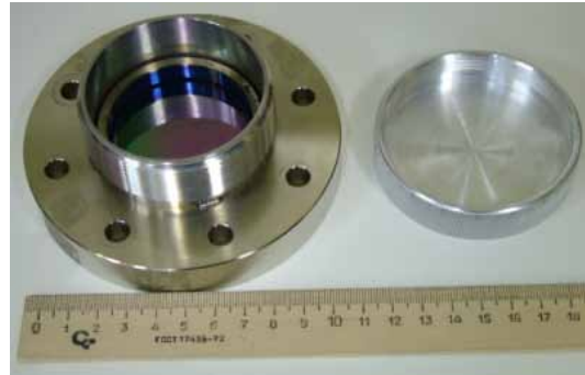
Fig. 5. GaAs high-vacuum window design.
