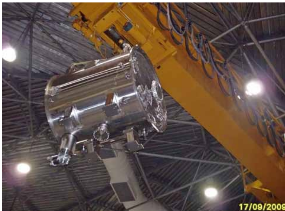
Fig. 33: Moving the upgraded shifter with a field of 7.5 T to the LSU-CAMD storage ring.
