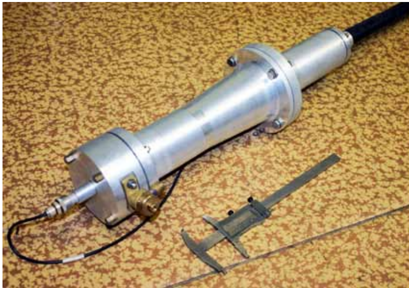
Fig. 4. High-voltage wideband load with a build-in divider.
