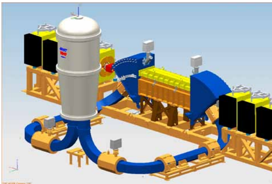
Fig. 1. 3D view of 2-MeV electron cooling installation.
