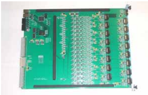
Fig. 4. The electron module of the 16-channel shaper-digitizer in VME standard and the electron module of the concentrator in VME standard.
