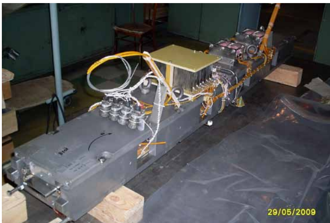
Fig. 35: Magnetic system of the 119-pole wiggler with a field of 2.2 T and period of 31 mm for the ALBA-CELLS storage ring (Spain).
