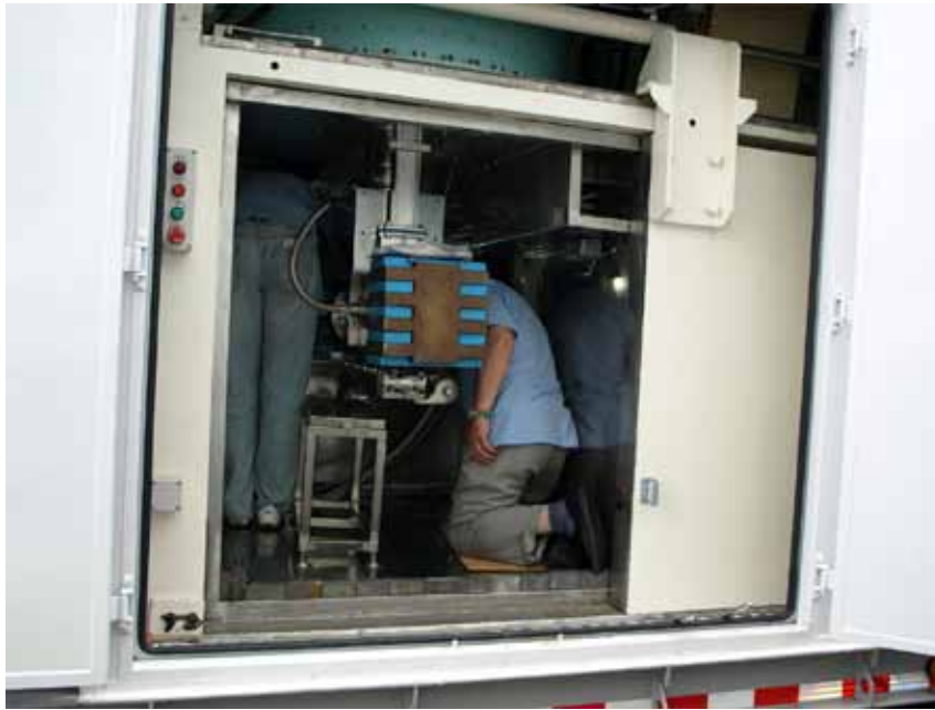
Fig. 2: Assembling of vacuum system of mobile accelerator.
