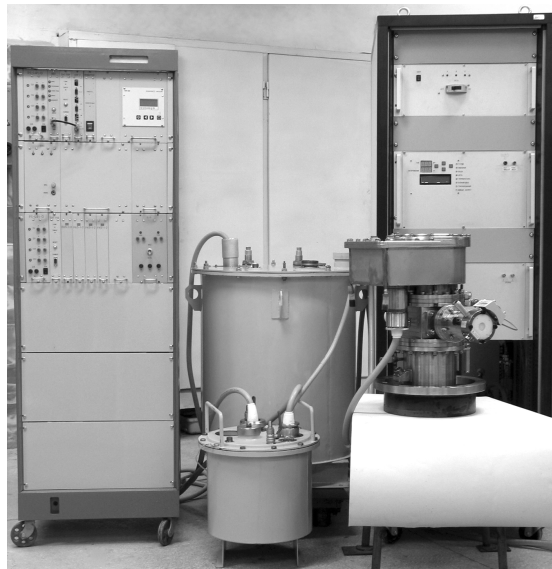
Figure 2: General view of the power supply unit for the electron-beam welding devices developed at BINP.
