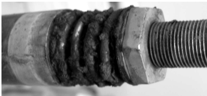
Figure 6: High voltage load element after 6-month operation in water.
