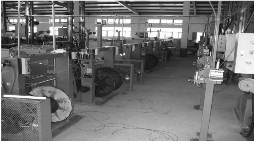
Figure 8: Pay-off and take up facilities in “Salipt” Company, Dongguan city, China.
