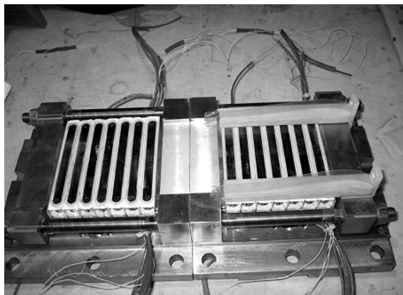
Figure 38: Assembly of the “short” prototype of the multipole wiggler with a period of 30 mm and magnetic field of 2.2 T for the ALBA-CELLS storage ring (Spain).
