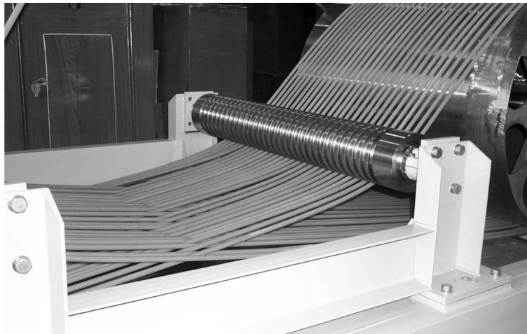
Figure 5: Cable wire bar of 36 \text{ mm}^2 cord section.
