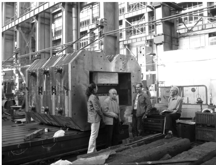
Figure 43: Iron yoke of the radiation-resistant H-type dipole magnet.
