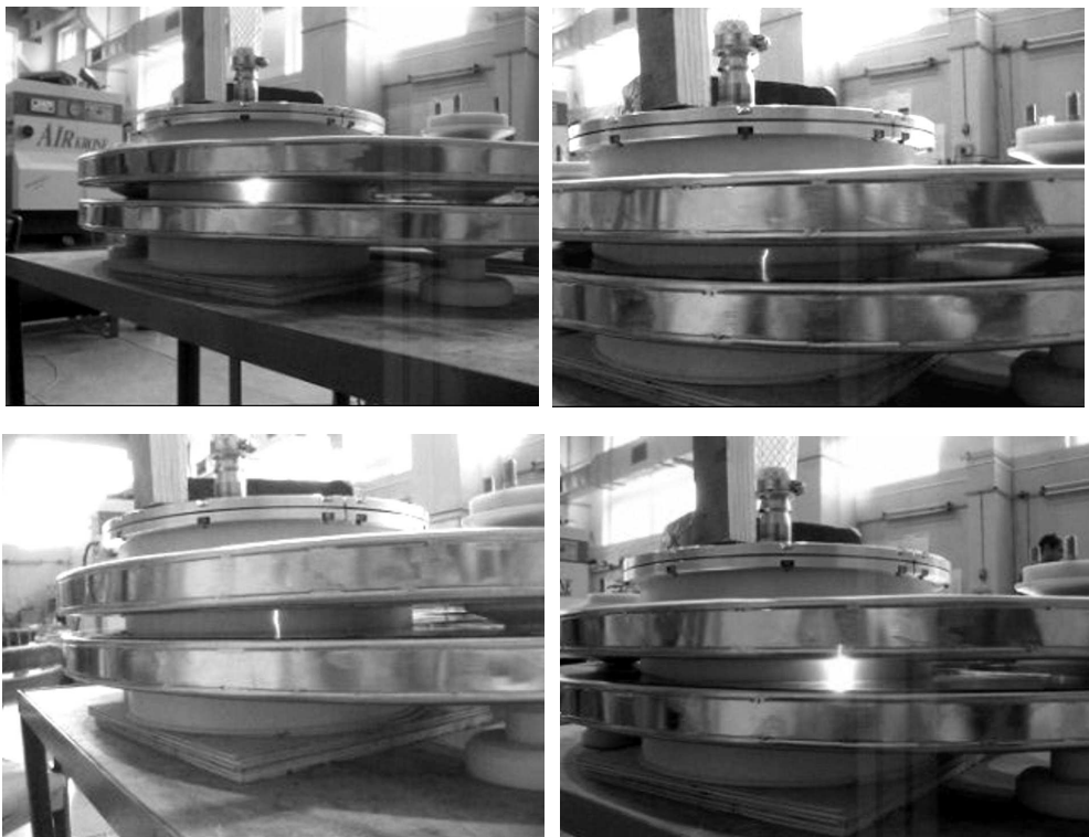
Figure 2: Photos of breakdowns between two sections at voltage of the order of 22 kV.
