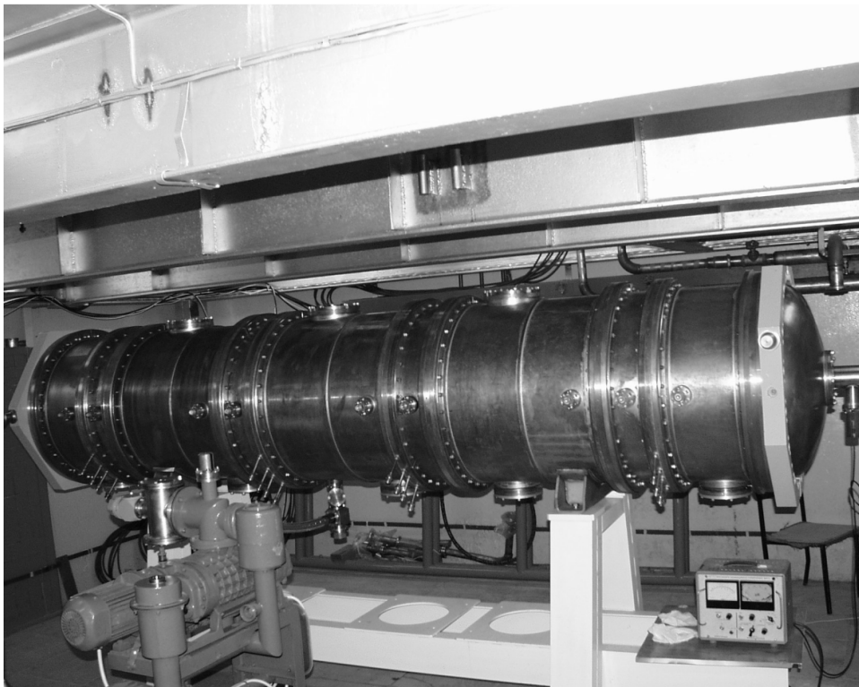
Figure 2: Mounted accelerating structure.
