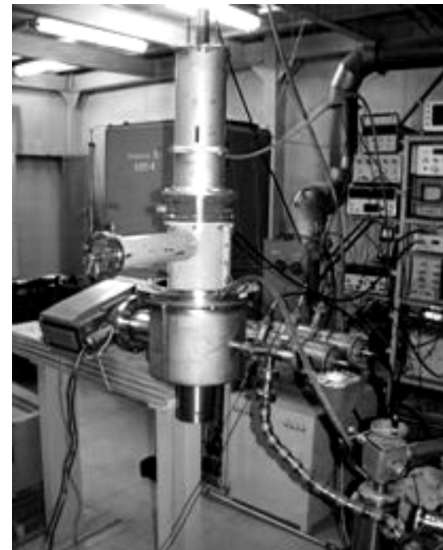
Figure 3: Stand for tests of power leads.
