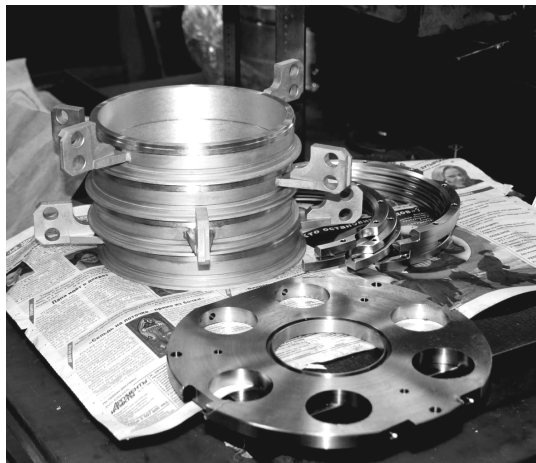
Figure 10: Details of the transverse feedback cavity.
