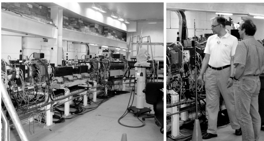
Figure 17: Mounting the booster synchrotron for Duke University.
