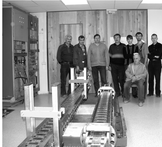
Figure 19: The first permanent magnet damping wigglers for Petra-III on the magnetic measurement bench.
