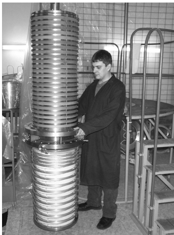
Figure 1: 1MV glass-ceramic feedthrough insulator.
