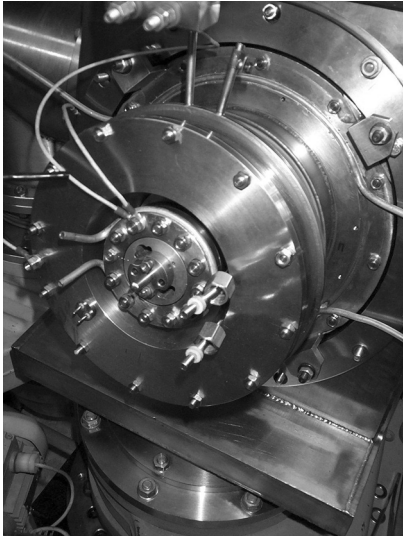
Figure 3: The flange variant of H-source.
