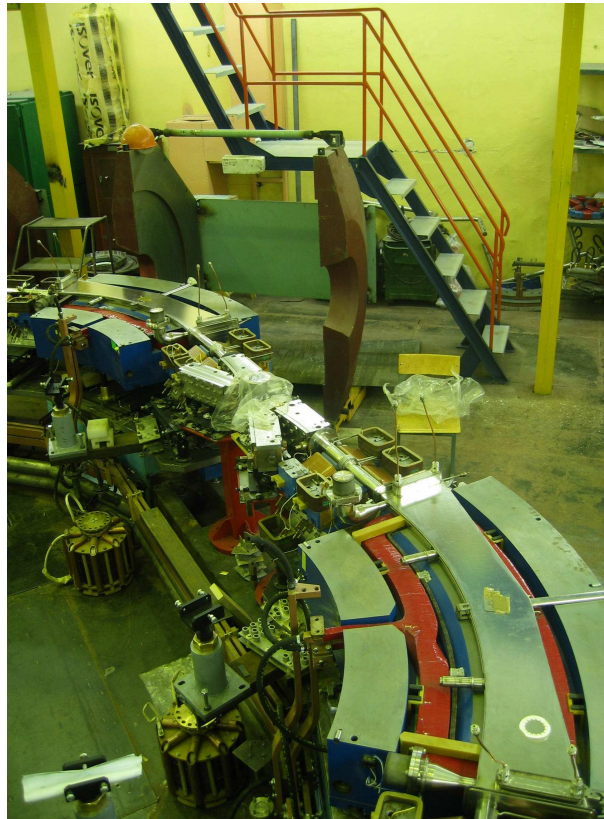
Figure 2: Vacuum chamber of bending magnets in connection with vacuum chamber of injection drift
