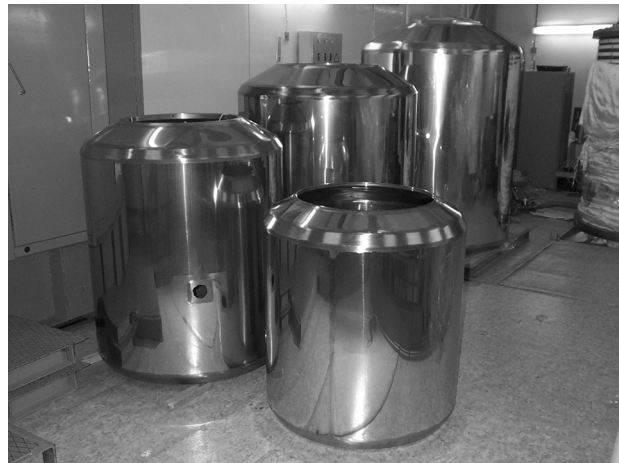
Figure 2: Electrodes of the high voltage accelerating gaps.
