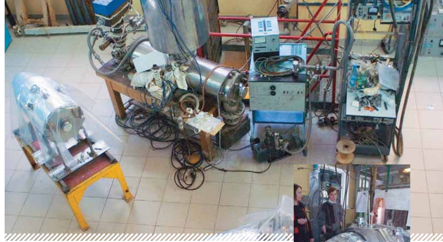
Superconducting solenoids operate at a very low temperature; therefore, each unit of a solenoid has a buffer volume of 200 liters for storage of liquid helium (its temperature is 4°K or — 269°С)
