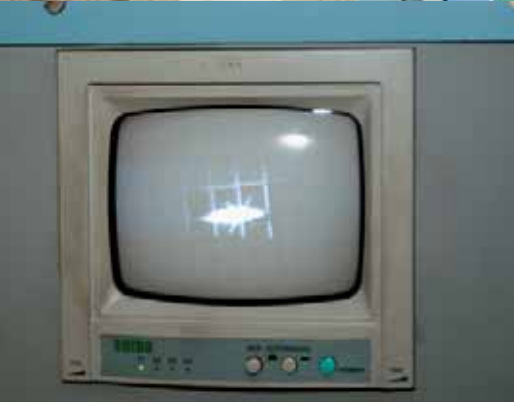
The monitor screen displays the photon "track" from the particle beam moving in the accelerator
