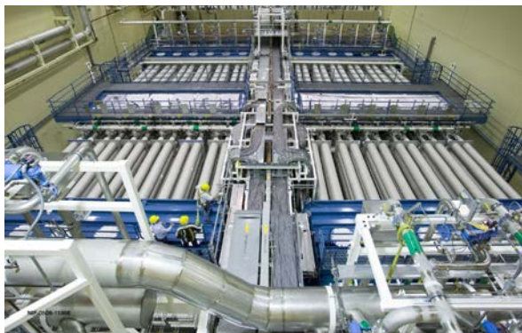
FIG. 10.38. NIF main amplifier. Taken from Refs [10.129, 10.130].
