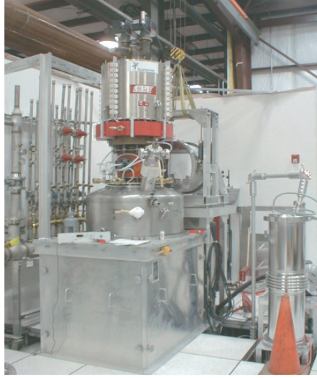
FIG. 6.83. The CPI 1 MW, 110 GHz gyrotron installed at General Atomics for heating the DIII-D tokamak (photo courtesy of John Lohr, General Atomics, USA). See also Ref. [6.272].
