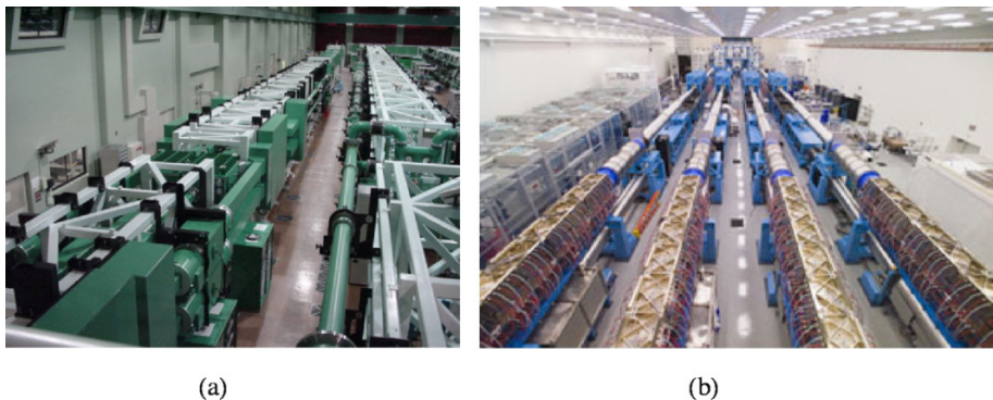
FIG. 10.31. (a) 10 kJ/10 ps LFEX laser; (b) 5 kJ/10 ps OMEGA-EP laser. Taken from Ref. [10.118].
