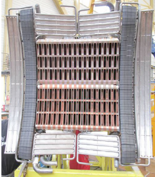
FIG. 6.48. Front face photograph of the Tore-Supra ITER prototype PAM launcher which is a quadrant of the proposed antenna for ITER.
