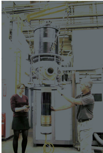
FIG. 6.86. A 2 MW, 95 GHz gyrotron at CPI. Reprinted from Ref. [6.277]. Copyright (2011) by the World Scientific Publishing Company.
