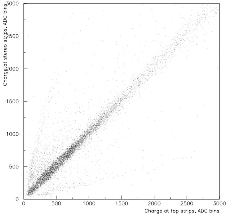
Figure 6: Correlation between cluster charge in top and in bottom layers.
