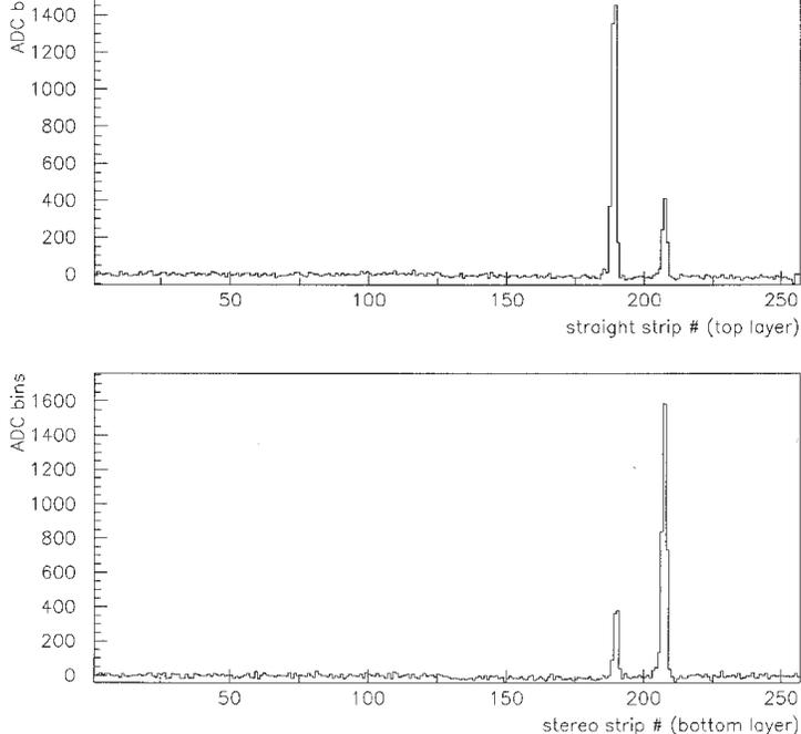
Figure 4: Typical signal from charged particle. Response of top and bottom layers is shown.
