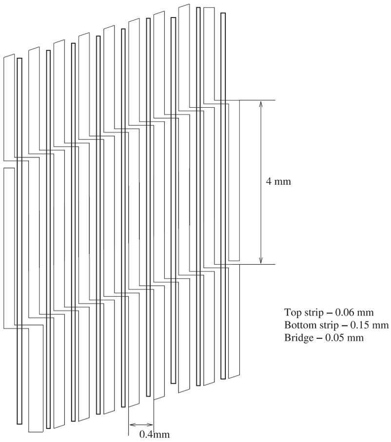
Figure 1: Schematic view of the PCB layout.
