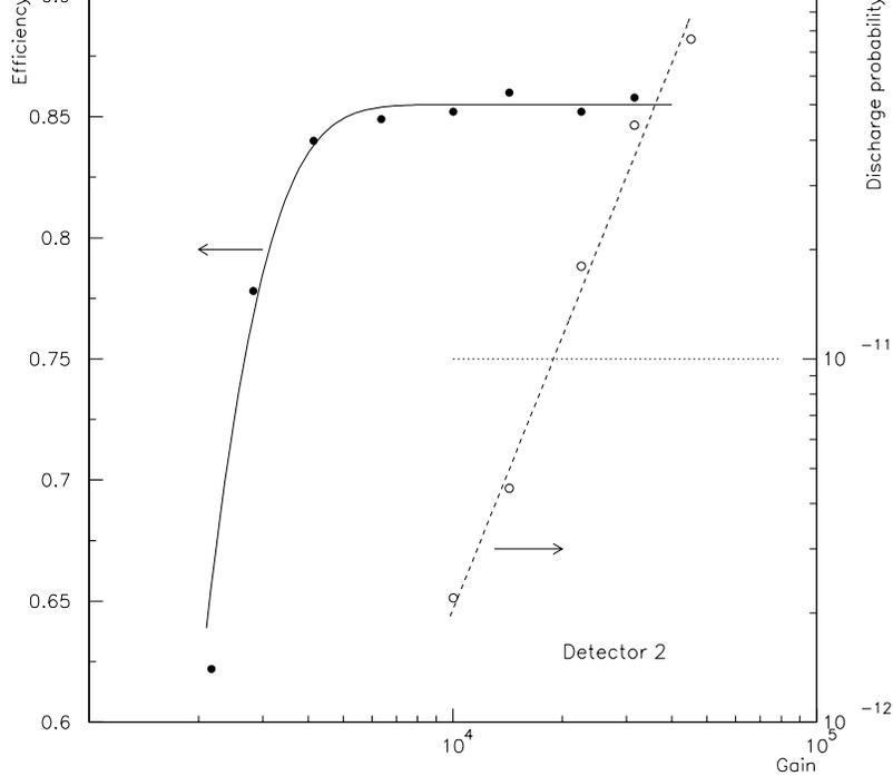
Figure 9: Dependence of efficiency (left scale) and discharge probability per incident particle(right scale) on gain. Dashed line is indicating the level of  $10^{-11}$  considered as a safe limit.
