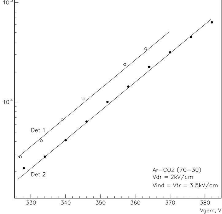
Figure 8: Dependence of gain on GEM voltage in two detectors.
