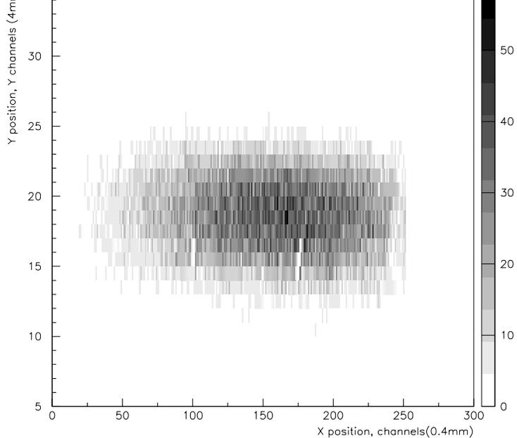
Figure 7: Beam profile measured at low intensity at detector 2.
