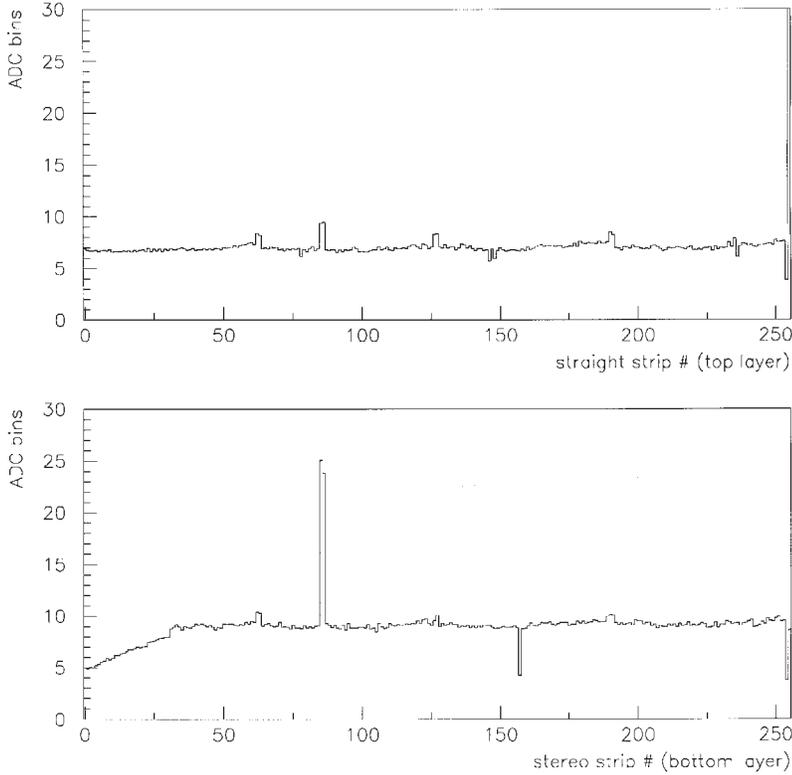
Figure 3: Noise values (sigma of gaussian fit) for all channels of the detector.
